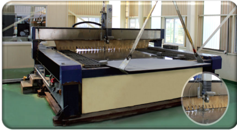
▲ WATER JET CUTTING M/C
