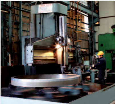
Vertical Lathe & Turning Machine • Max. working dia. : 4,500 mm
