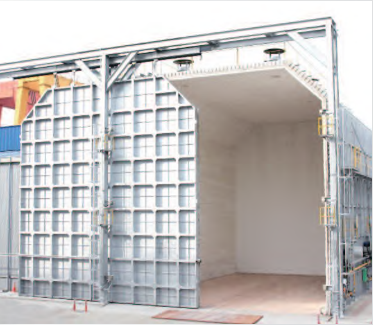
Annealing furnace (Max. Temperature : 1,150 °C)
