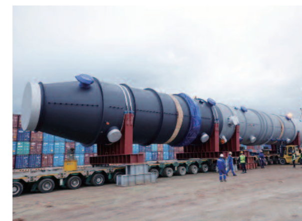
3-CAR Heat Exchanger (SA240-304H,SA516-70N,SA516-70 / SA213-304H,SA213-T11 / SA179) • Client : Zhejiang Petroleum & Chemical Co., Ltd./ China (2018) • Size(mm) : (23,95,25/40,20)T X ID 4,444 X L 40,730 / 605 Ton
