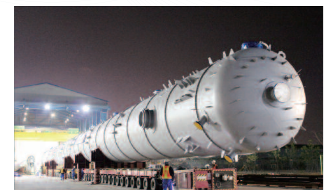
Propylene Fractionator (Big Tower, SA516-70N) • Client : Samsung Total Petrochemicals Co., Ltd/ Korea (2013) • Size(mm) : (60+1.5)T X ID 4,100 X L 98,600 / 776.7 Ton
