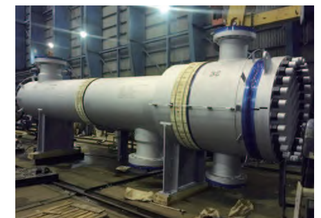
Modified 'D' Type Heat Exchanger (SA387-22CL2+316L Clad / SA336-F22CL3 + 347 SS Depo. / SA213-TP321) • Client : Bangchak Corporation/ Thailand (2018) • Size(mm) : 142(Th'k on channel)T X ID 1,050 X L 8,408 / 34 Ton
