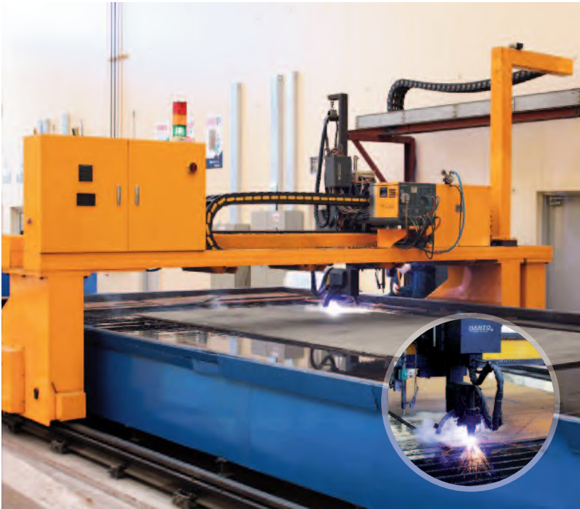
CNC Plasma Jet Cutting Machine • Max. Cutting Thickness : 80 mm
