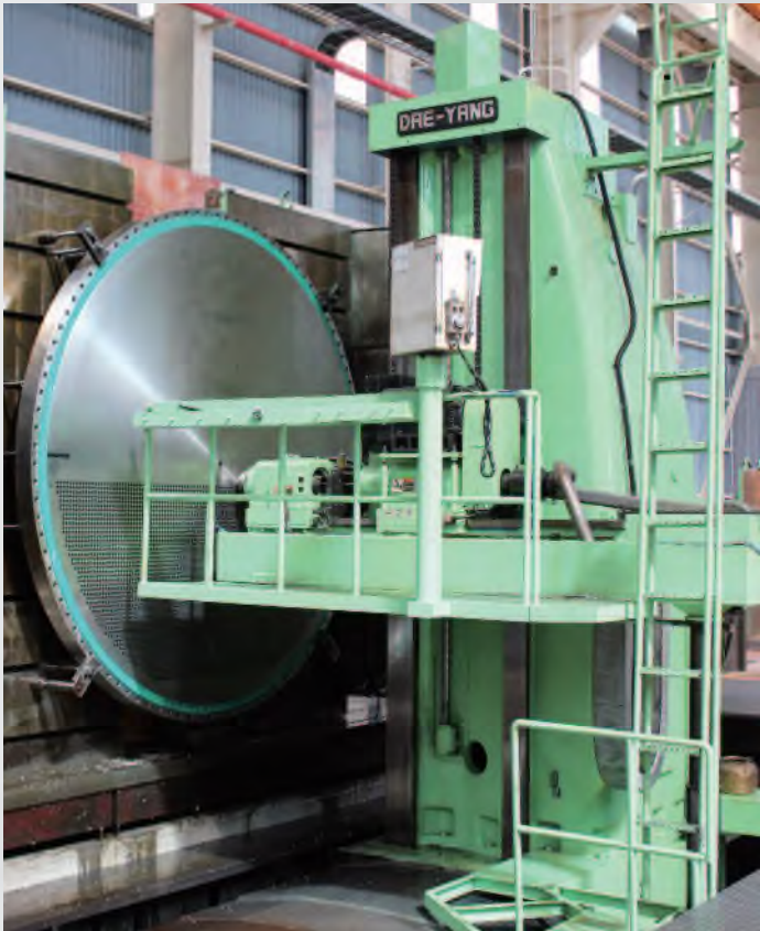
B.T.A & deep hole drilling machine • Max. working dia : 6,000 mm, Max. drilling thickness : 1,000 mm
