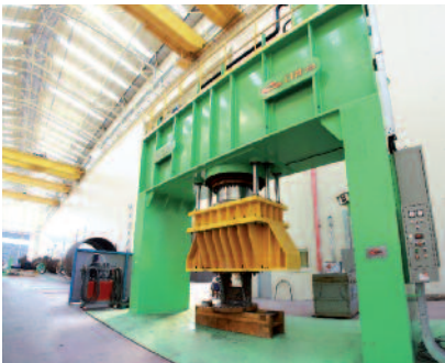
Hydraulic Press • Pressing capacity : 1,500 Ton
