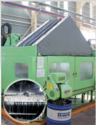
CNC Drill Machine (Drill Master) • Max. working dia : 3,000 mm, • Max. drilling thickness : 400 mm
