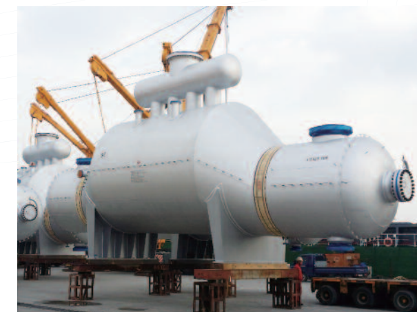
Titanium Heat Exchanger (SA516-70N / SB338-2) • Client : China Prosperity Petrochemical Co., Ltd./ China (2015) • Size(mm) : (55/48)T X ID 4,850 X L 14,803 / 113.5 Ton
