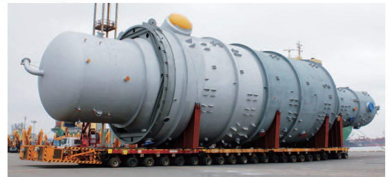
Vacuum Column (SA204-AN+SA240+316 Clad) • Client : Oman Oil Refineries and Petroleum Industries Company/ Oman (2015) • Size(mm) : (31+3)T X ID 10,000 X L 43,750 / 439 Ton
