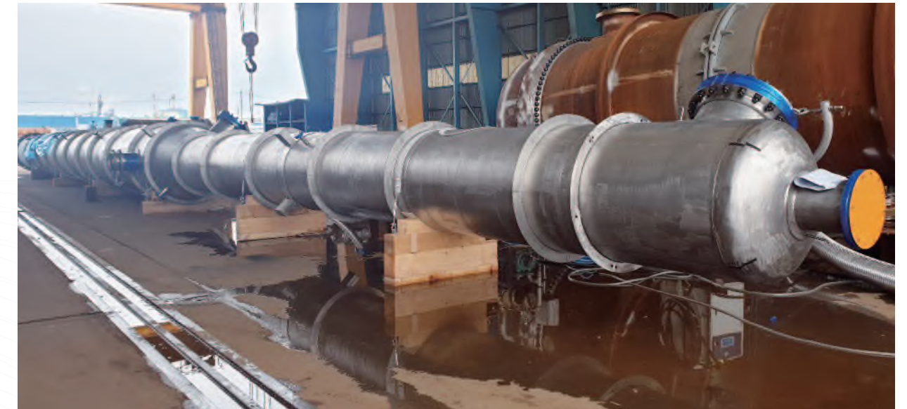
Zirconium Column for Acetic Acid Plant (B551-R60702) • Client : Lotte BP Chemicals/ Korea (2019) • Size(mm) : 10T X ID 1,115/1,600 X L 39,900 / 17 Ton
