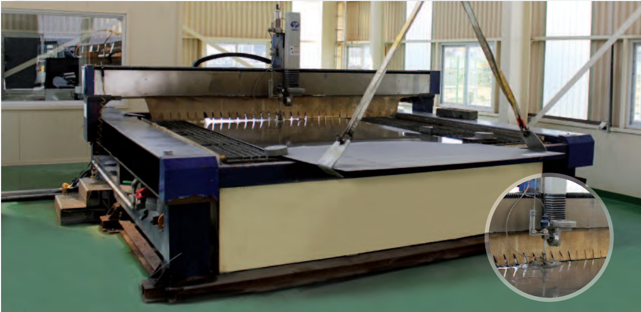
Water Jet Cutting Machine • Max. Cutting Thickness : 100 mm
