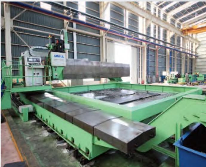
CNC Drill Master • Max. working dia : 5,000 mm • Max. drilling thickness : 100 mm
