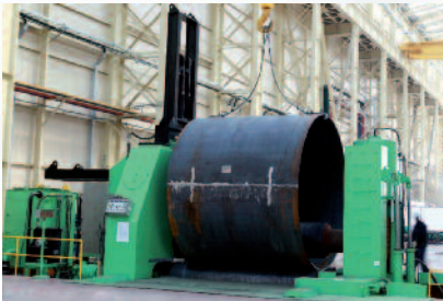
Bending Roller • Max. thickness : 90 mm
