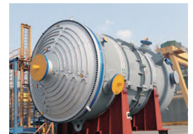
Oxychlorination Reactor (SA516-70N/B163-N02200)
