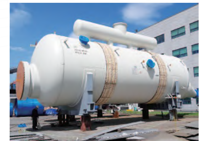
Chain Type C3 Chiller (SA240-304/304L / SA213-304/304L) • Client : BP Tangguh LNG/ Indonesia (2018) • Size(mm) : (29/67)T X ID 5,100 / 2,070 X L 21,630 / 422.6 Ton
