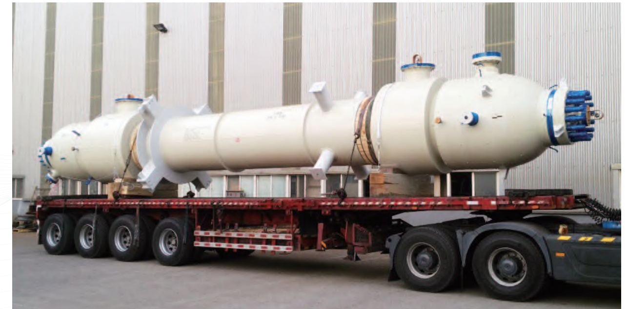
Carbamate Condenser (Advanced High-Alloy Duplex Material) for Urea Process • Client : P.T. Petrokimia Gresik/ Indonesia (2017) • Size(mm): (14/127)T x ID 1,300 / 1,360 x L 14,300 / 56 Ton
